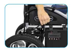
Note: When parked on a sloped surface, the brake lever must be pushed forward, otherwise the wheelchair will lose control and result in personal injury.
