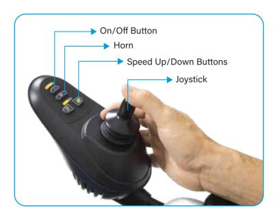
The **On/Off-Button** controls power to the wheelchair. Don't use the On/Off-Button to stop the wheelchair unless some emergency occurs, as doing so may cause premature wear of the drive components.
