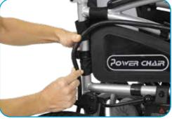
7. Connect the wiring harness plug of the controller with the socket harness socket from the batteries.
