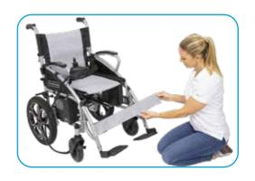
11. Adjust the height of the footplate, unload the safety nut on either side of the footplate, pull out the bolts, slide up and down the telescopic tube, position at a comfortable height, then insert the bolts, and lock the nut.
