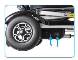
Assemble the power block and power cord. Connect the power block to the scooter, and plug into a standard wall outlet.
