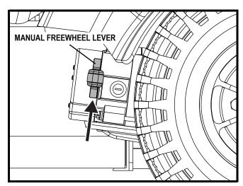
Figure 5. Drive Mode (Drive Engaged)
