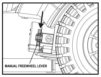
Figure 4. Freewheel Mode (Drive Disengaged)
