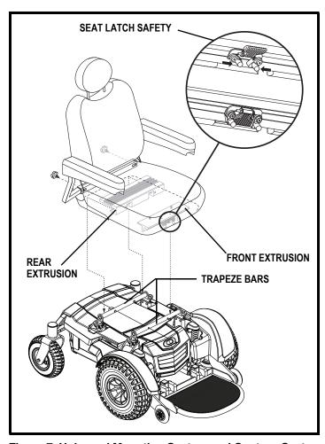
Figure 7. Universal Mounting System and Contour Seat
