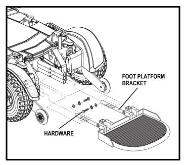
Figure 15. Foot Platform Adjustment
