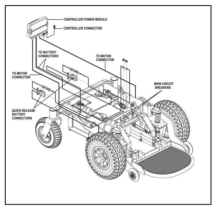
Figure 3. Quantum/Jazzy 1450 Series Electrical Components
