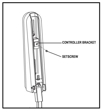
Figure 14. Underside of Armrest
