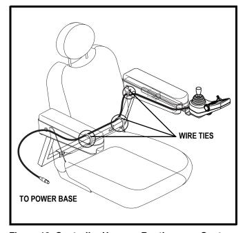
Figure 10. Controller Harness Routing on a Contour Seat
