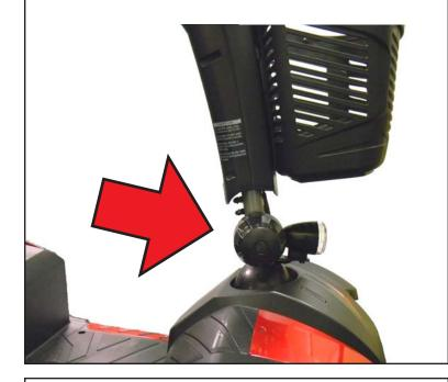
If equipped (DLX models), connect the rear light harness on the rear shroud to the main cable 5. on the base of the scooter.
