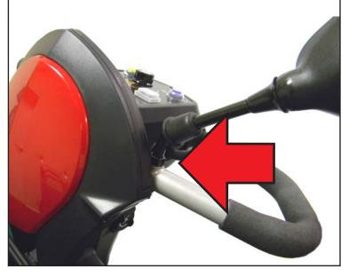
**2.** Before use, make sure that the scooter's yellow freewheel mode lever is in the "drive" position.
