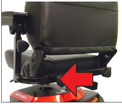
**9.** Attach the front basket by aligning the bracket on the tiller with the mounting holes on the basket. Then push down to secure in place.
