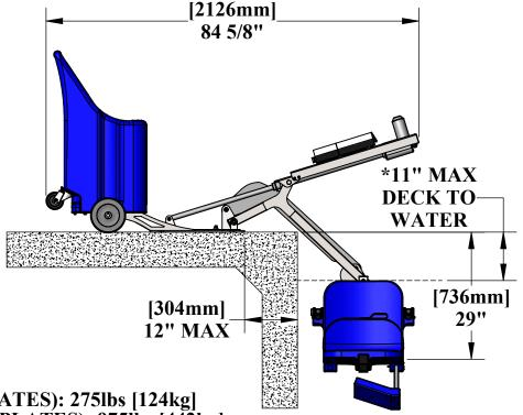
PRODUCT WEIGHT (NO PLATES): 275lbs [124kg] PRODUCT WEIGHT (WITH PLATES): 975lbs [442kg] MAX WEIGHT CAPACITY: 350lbs [160kg]
