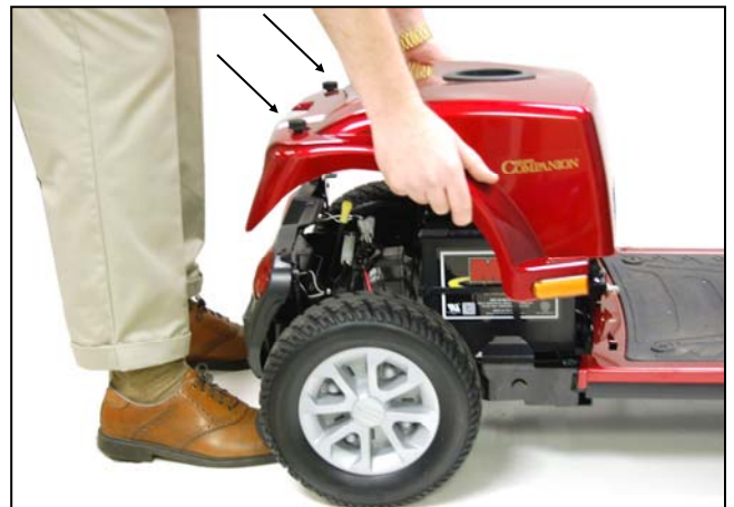
FIGURE 16. REMOVING THE REAR SHROUD
