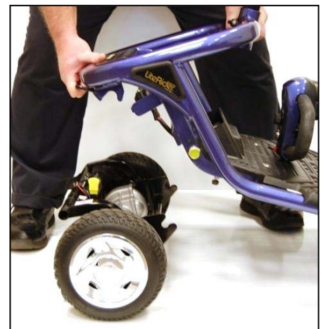
Figure 18. Lifting the Frame
