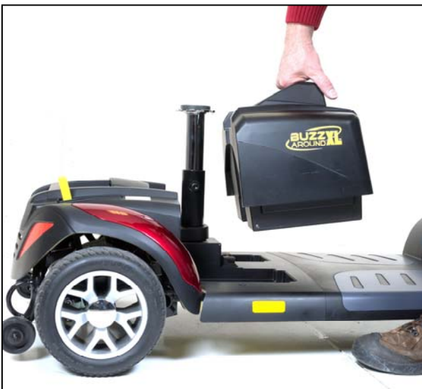
Figure 21. Battery Pack Installation
