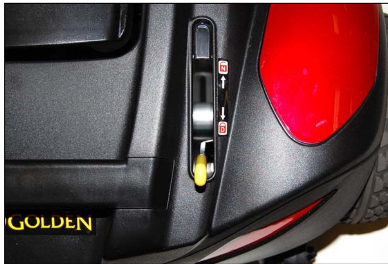
Figure 11: Freewheel Lever (Drive Position)
