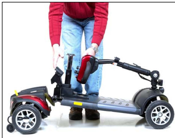
Figure 17. Separating the Drivetrain and Frame
