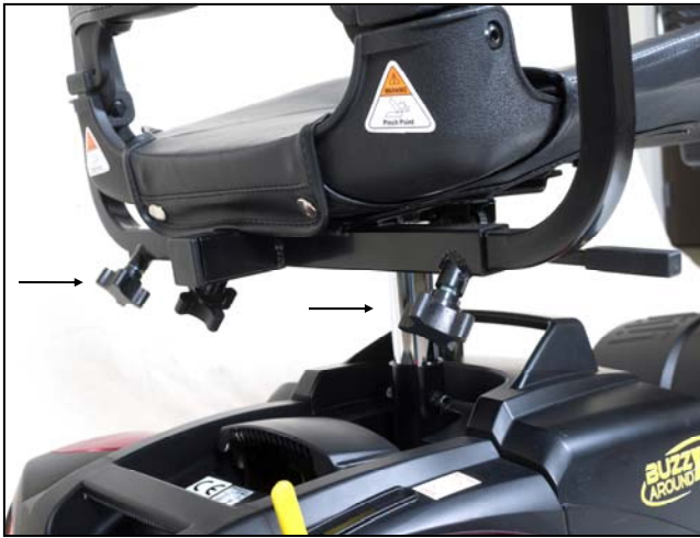
Figure 6. Armrest Width Adjustment
