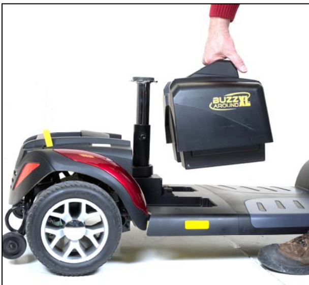
Figure 21. Battery Pack Installation
