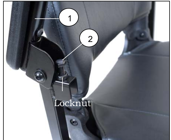
Figure 7. Armrest Angle Adjustment
