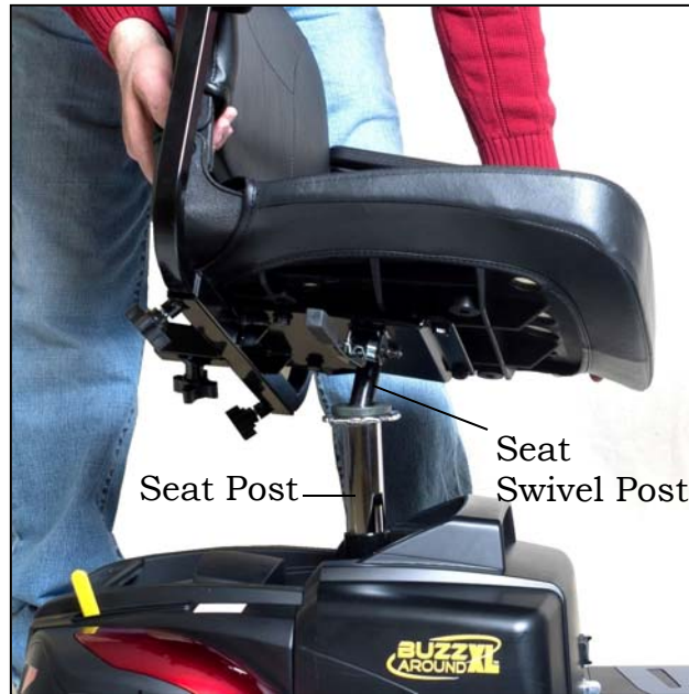
Figure 23. Installing the Seat
