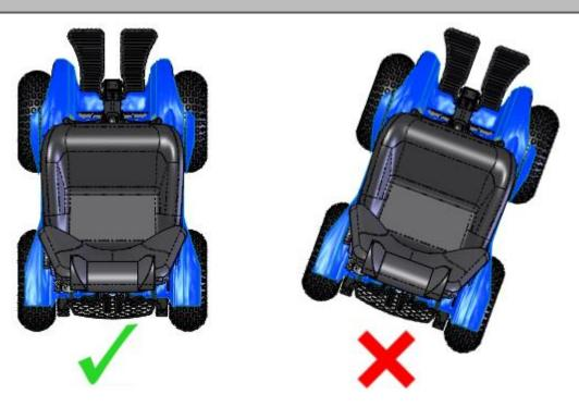
Figure 5 - Extreme X8 Correct and Incorrect Approaches to Obstacles
