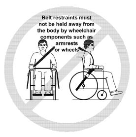
Figure 13 - Improper belt restraint fit
