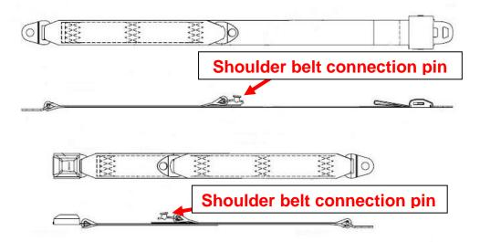
Figure 25 - The Wheelchair Anchored Pelvic Belt
