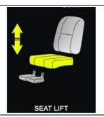
Displays the sections of the chair currently selected for movement and a direction arrow
