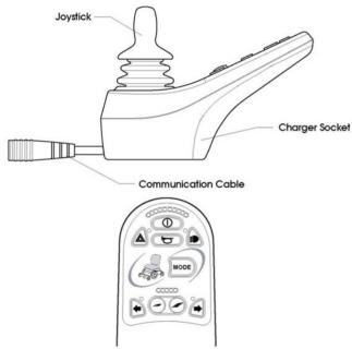
Figure 12 - LED Joystick Module
