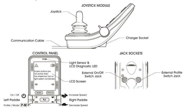
Figure 14 - CJSM2 Joystick Module
