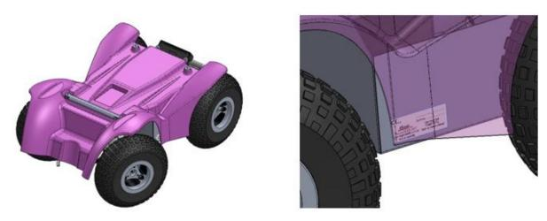
Figure 2 - Extreme X8 Serial Number Location
