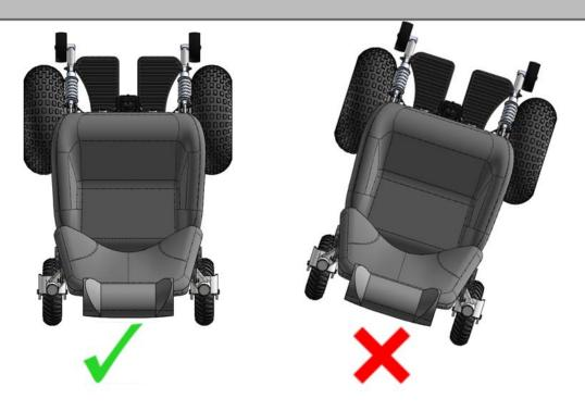
Figure 6 - Frontier V4 FWD Correct and Incorrect Approaches to Obstacles
