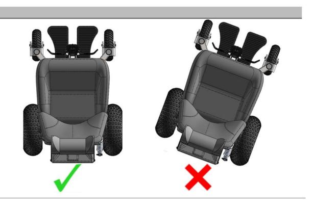
Figure 7 - Frontier V4 RWD Correct and Incorrect Approaches to Obstacles
