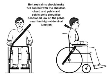
Figure 14 - Proper belt restraint fit
