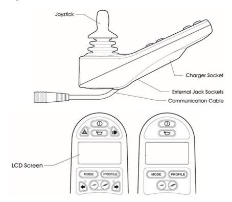
Figure 13 - LCD Joystick Module (with and without light buttons)
