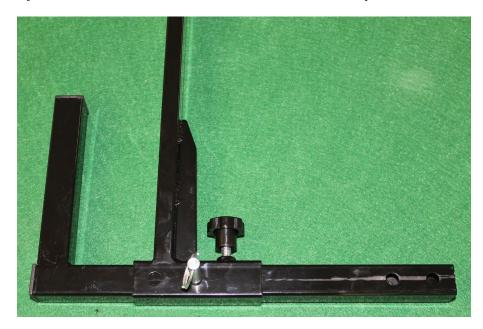
Slide the Mount Bar into the receiver under the seat. Pin this in place with a clevis Pin using the first or second hole.
