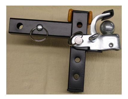
9. Remove the smaller Clevis pin from the receiver. Adjust the height according to your preference. Re-insert the smaller Clevis Pin. Do not forget to include the small, flat shelf piece (pictured below). This keeps the ball hitch from hanging.
