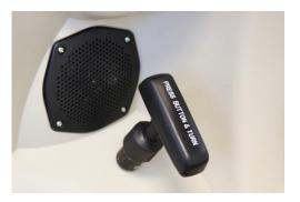
To activate the emergency brake, first start by depressing the foot pedal to alleviate tension from the brake lines. Keep the brake pedal depressed while activating or releasing the emergency brake. Pull the handle out towards you while the handle is in the vertical position to activate.
