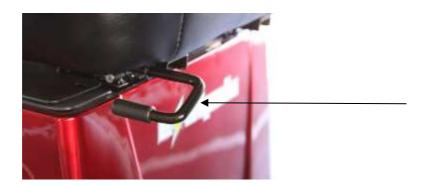
2. Locate the reclining seat lever located on side of seat.
