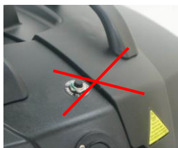
(Incorrect) Not securely locked
