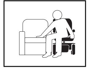
Figure 8. Recommended Transfer Position
