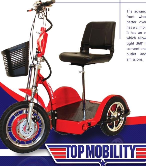
The advanced powerful 750 Watt front wheel-motor provides a better overall performance, and has a climbing angle of 17 degrees. It has an excellent turning radius which allows the user to make a tight 360° turn. It plugs into any conventional 110-volt household outlet and has zero exhaust emissions
