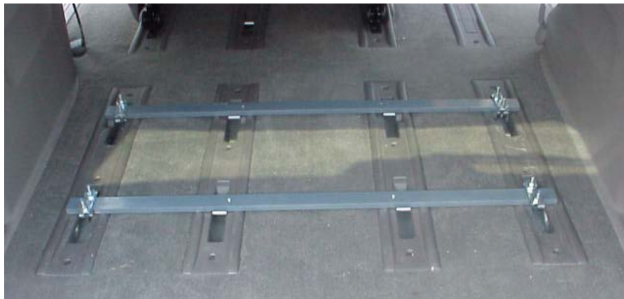
Example: Mounting Bars Installed
