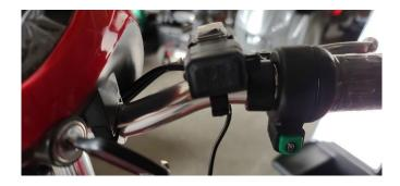
1. Assemble the nut into the Handlebar Mounting Clamp. Slide the USB Port Housing onto the mounting clamp. **NOTE:** This figure below does not show the USB Housing <u>FULLY</u> slid onto the mounting clamp.
