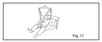
7) Pull lift away from bed. Lower lift (and patient) to a suitable minimum height for transferring. The patient should not be pushed/pulled by the sling handles. Pulling the patient with sling handles could result in moving patient's weight outside the lift base and tipping the lift, especially in the high position.
