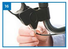
too tight, use your fingers or pliers to turn the larger locking nut counterclockwise until loosened. Then use fingers or pliers to turn barrel adjuster nut clockwise a half at a time until the brake functions as expected. Then turn the locking nut clockwise until it presses tightly against the housing to prevent the barrel adjuster nut from loosening.
