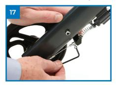
cable length, tighten the set screw by turning clockwise. You may have to repeat adjustment a few times to get it right.
