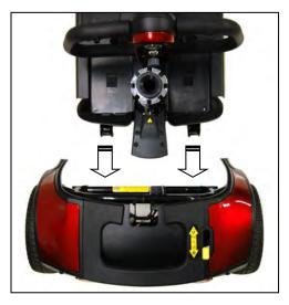
Figure 19. Drivetrain Alignment
