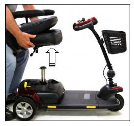
Figure 14. Removing the Seat
