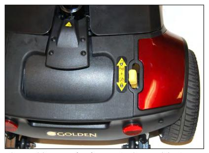
Figure 11: Freewheel Lever (Drive Position)
