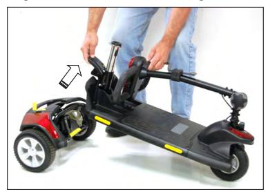
Figure 17. Separating the Drivetrain and Frame
