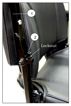
Figure 7. Armrest Angle Adjustment
