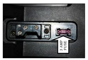
Figure 26. Under Battery Pack
