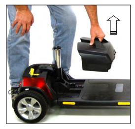
Figure 15. Removing the Battery Pack
