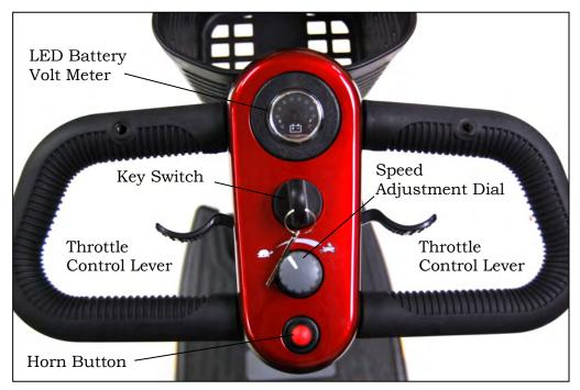
Figure 5. Buzzaround XL<sup>TM</sup> Delta Tiller Control Panel
