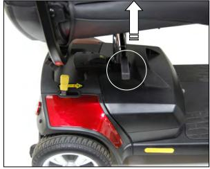
Figure 8: Seat Rotation Adjustment
