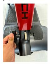
4.Put your hand on the backrest bracket center beam part, and lift it up until the seat limit pin pops out, at the same time you can hear the "crack "sound, then try to push the seat forward to make sure the seat no longer being folding.
