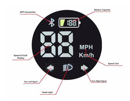
Turn on the power, then the display screen will show the battery remaining power percentage. At the same time, we can judge the battery power through the indicator light color.
