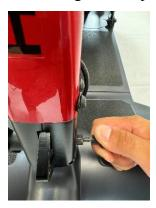
3. After raising the steering handle and adjust it to a comfortable angle slightly, then tighten the locking bolt. (The locking bolt is located the opposite of the folding limit pin).
